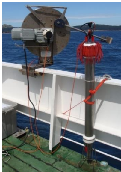
Figure 1.6. MSS 90 multiparameter high resolution profiler (ISW Wassermesstechnik and Sea & Sun Technology GmbH, Germany) for the measurement of microstructure turbulence in aquatic environments.
